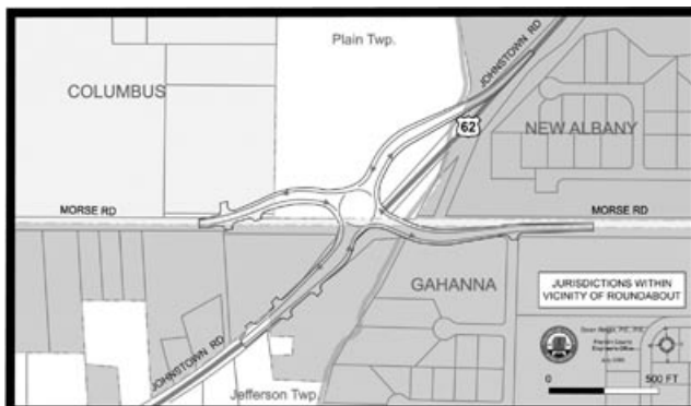
Diagram of the proposed modern roundabout at U.S. Route 62 and Morse Road in northeast Franklin County.
