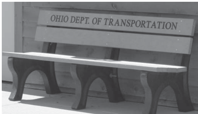
Benches and picnic tables at the U.S. 23 southbound rest area in Marion County are made from recycled milk cartons.
