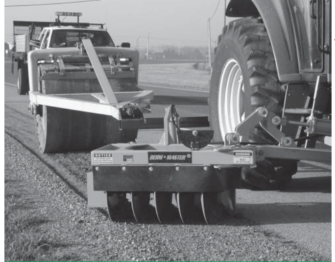
Attached to a mowing tractor, the berm recovery device can be used to recover berm stone knocked out of place and move it back into position along the edge of a roadway.
