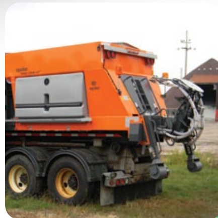
The EPOKE hopper, left, is interchangeable with the usual dump truck bed.
