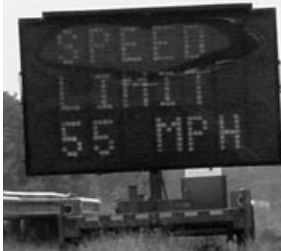
This portable, changeable message board along the I-71 work zone in Richland County has an attached speed trailer warning speeders to slow down and reminding all motorist of the reduced speed limit.
