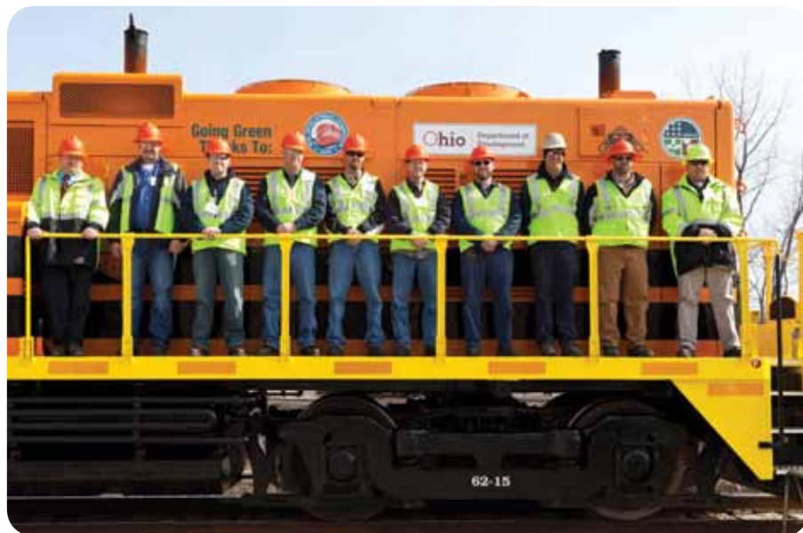
Genesee & Wyoming’s new “Gen-Set” locomotive. The shop crew, pictured, gutted a 1950’s-era yard switcher and rebuilt it from the frame up at G&W’s locomotive shop in Coshocton.
