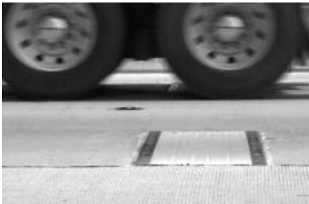
Embedded Automated Traffic Recorders, such as this one, capture important information on vehicles using Ohio's roadways.
