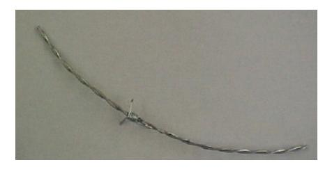
The permissible variation from the nominal diameter of the wire, for both line wires and barbs, for all types, shall be  $\pm 0.005$  inches.
