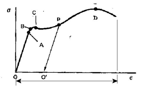
This graph above is a typical STRESS - STRAIN curve for a steel material.
