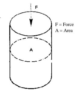
Example: A Force of 600 lbs is applied to a 1/4" diameter rod what is the STRESS in Psi?
