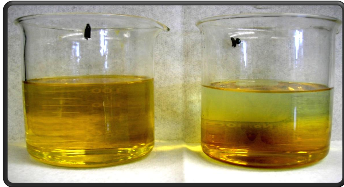
Image 1: Represents the visual appearance of the bio-diesel fuels when switching the order of component addition.
