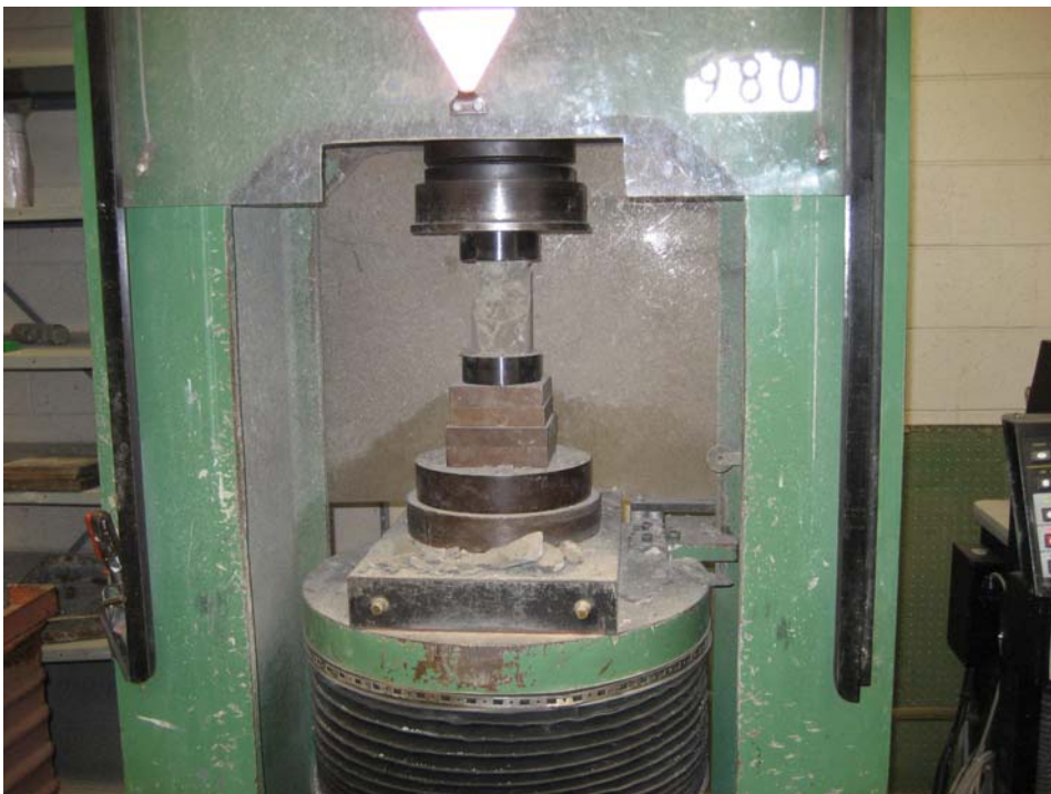
PHOTO 9: Compression testing of the cores
