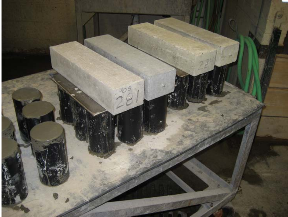
PHOTO 4: Restrained Cylindrical Specimens
