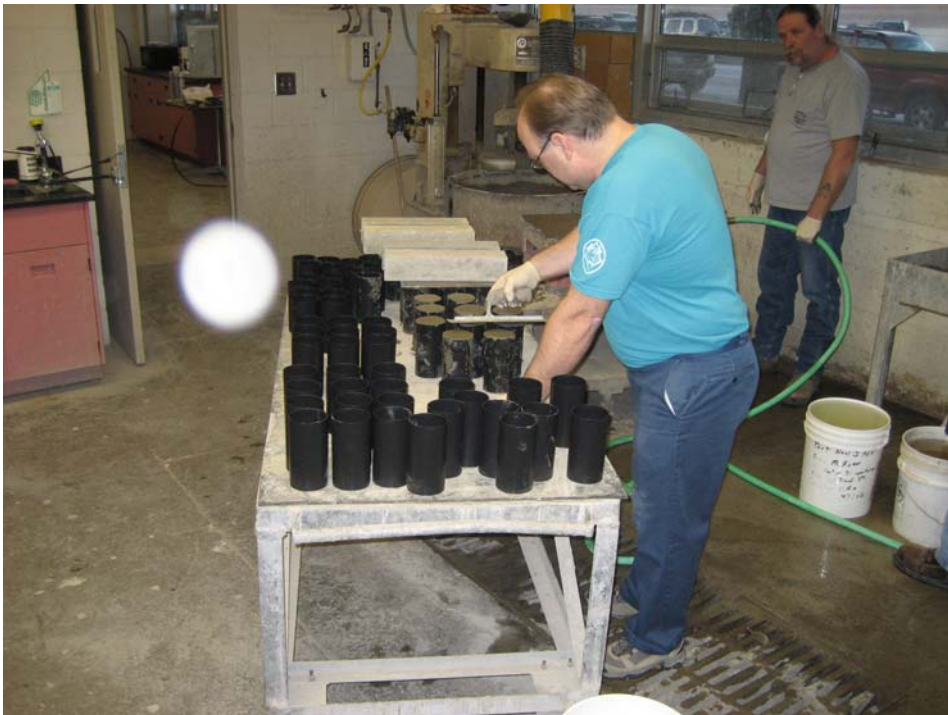
PHOTO 3: Setting up of the Restraining system to prevent expansion
