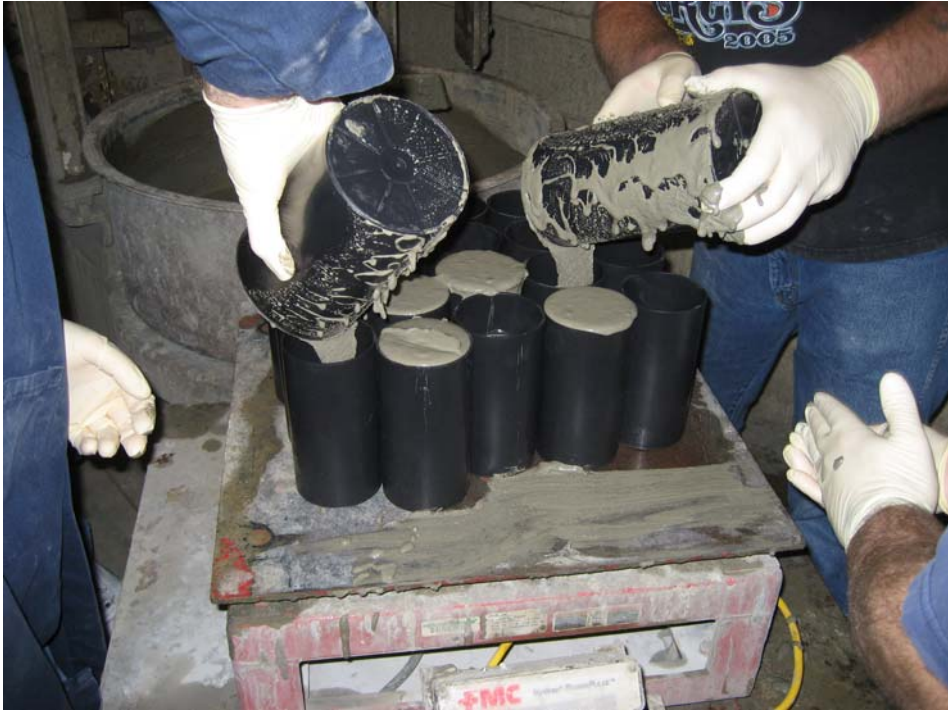
PHOTO 2: Molding of the Cylindrical Specimens and the table vibrator
