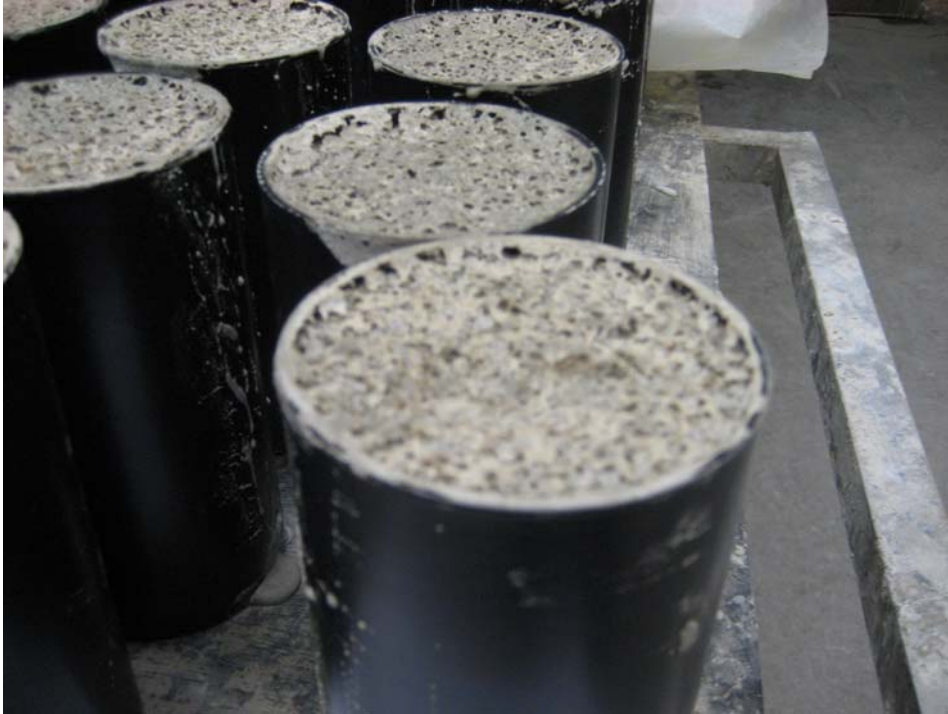
PHOTO 8: Shrinkage of W.R. Meadows – CG-86 Cylindrical Specimens
