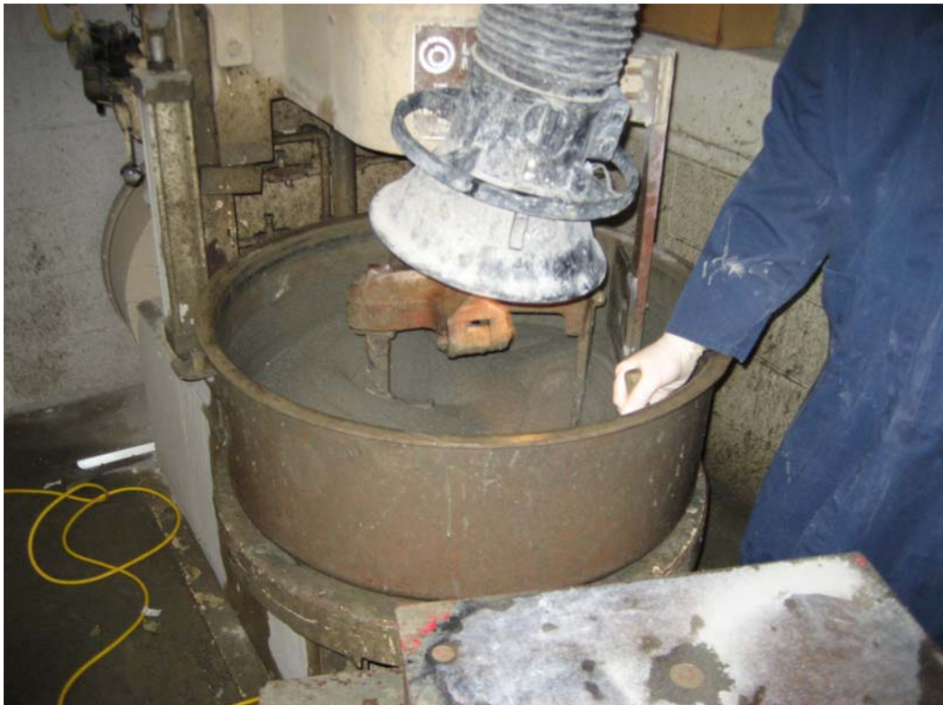
PHOTO 1: Mixing Operation of the Grout
