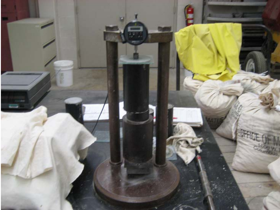
PHOTO 10: Extensometer setup to measure expansion/shrinkage of cylindrical specimens
