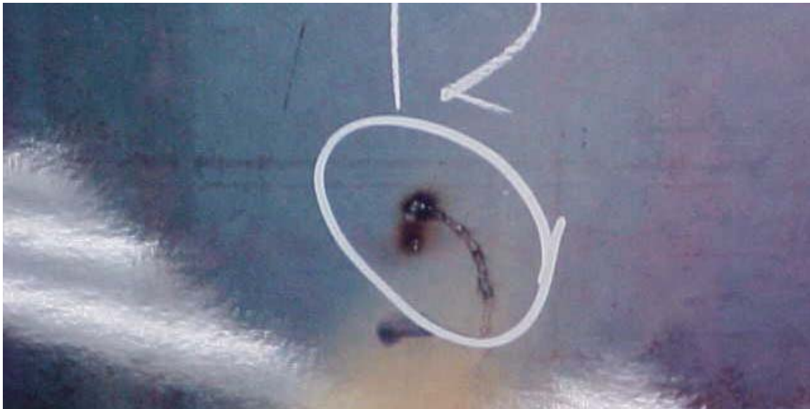
Example of an arc strike
