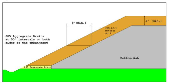
Place Bottom Ash on the prepared foundation in horizontal loose lifts not to exceed 8 inches (200 mm).
