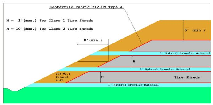
Place and compact a 1 foot (0.3 m) layer of natural granular material on a prepared foundation.
