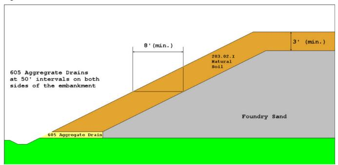
Place Foundry Sand on the prepared foundation in horizontal loose lifts not to exceed 8 inches (200 mm). Compact the lifts to a stable, durable condition with at least eight passes of a vibratory steel wheel roller. The roller shall have a minimum weight of 10 tons (9 metric tons) or its centrifugal equivalent. Compact lifts to 98 percent of the Supplement 1015.06 Test Section Method B Maximum Density.
