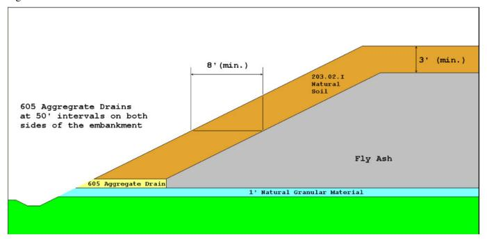
Place and compact a 1 foot (0.3 m) layer of natural granular material on the prepared foundation. Spread Fly Ash in horizontal loose lifts not to exceed 8 inches (200 mm). Compact Fly Ash at 3 percent below optimum moisture or dryer. Uniformly apply and evenly mix water into dry material. Disc and aerate wet material.
