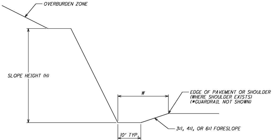
*\*Guardrail Required For All 3:1 Slopes and 4:1 Slopes With Safety Grading*
