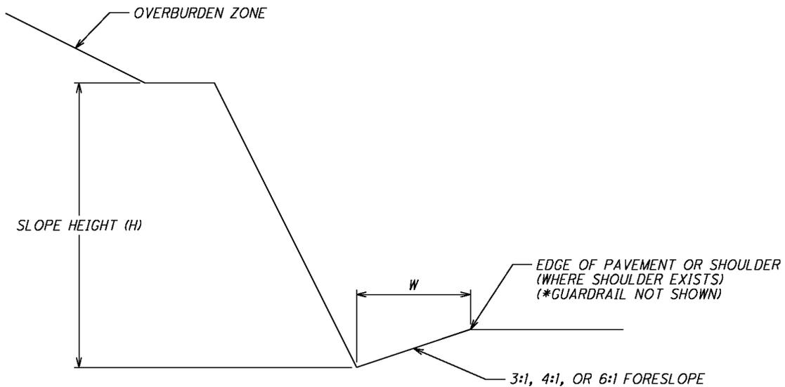
*\*Guardrail Required For All 3:1 Slopes and 4:1 Slopes With Safety Grading*
