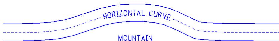
Horizontal curve data for simple curves is shown on the plan view. Horizontal curve data for spiral curves (where the curve radius is not constant) may only show the P.I. station, delta and degree of curve on the plan and profile sheet if the entire curve data has been shown on the schematic plan.
