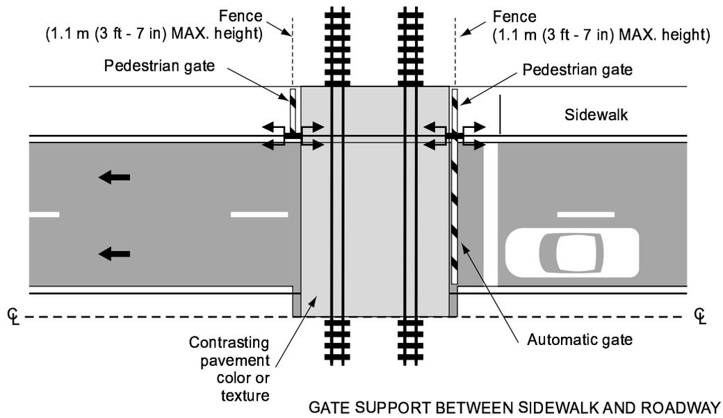
**Figure 10D-6. Example of Swing Gates**
