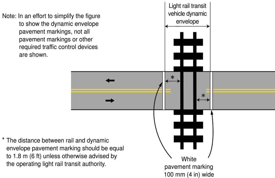
**Figure 10C-9. Example of Light Rail Transit Vehicle Dynamic Envelope Pavement Markings**
