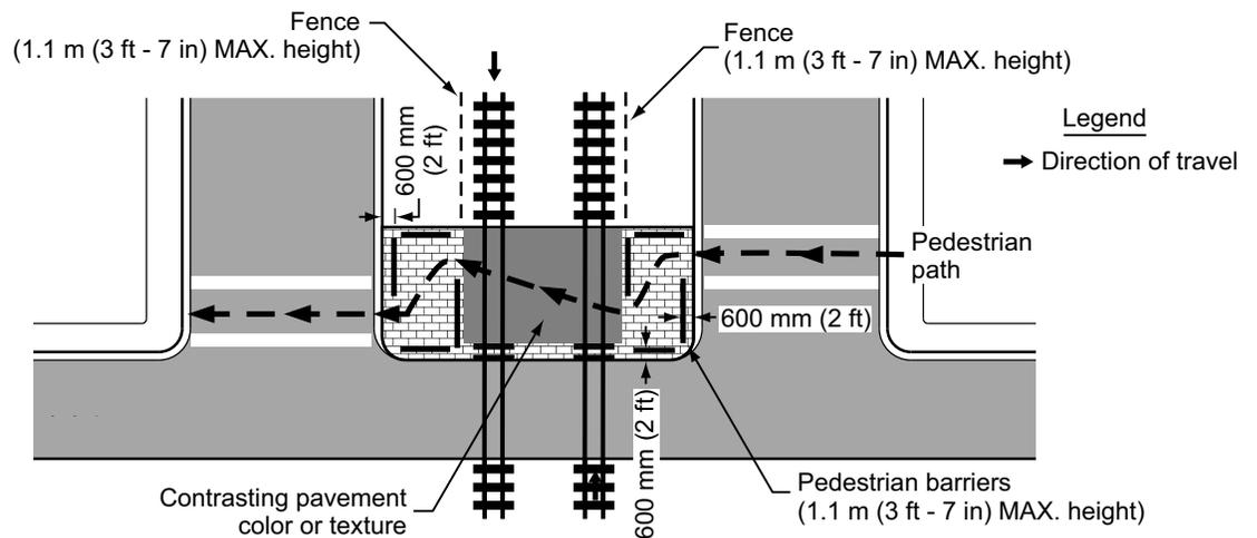
**Figure 10D-8. Examples of Pedestrian Barrier Installation at an Offset Nonintersection Light Rail Transit Crossing**
