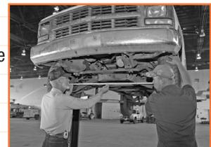
to make sure the vehicle is the proper test weight, then apply measurement stickers all over the exterior. These are used to measure speed and displacement on high-speed video and 16 mm film.
