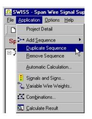
The span configuration and all data, excluding combination data, will be duplicated as the next available sequence number. This feature provides an easy way to compare multiple copies of the same span configuration with minor revisions in each one; such as changing the elevation differences or sag.
