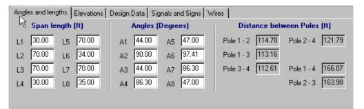
The length of each span segment is entered in feet. The span length is the horizontal distance from pole to pole, pole to bullring, or bullring to bullring depending on the span configuration. A number greater than zero must be entered for each length required in the configuration. A small value (0.1 foot) may be used for a span length attached to a pole to simulate the absence of the span segment.
