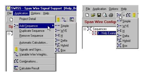
A graphic representation of the span configuration will appear in the window on the right side of the screen. Also, the sequence number and span type will appear in the left window under "Span Wire Configuration". Data may now be input for this span.
