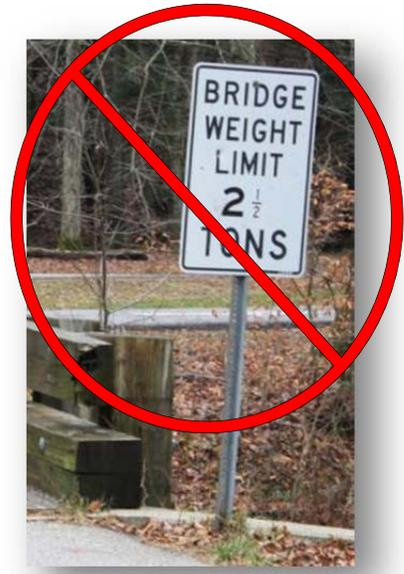
**Figure 15 - Bridge Must be Closed for loads less than 3T and fractions or decimals shall not be used.**
