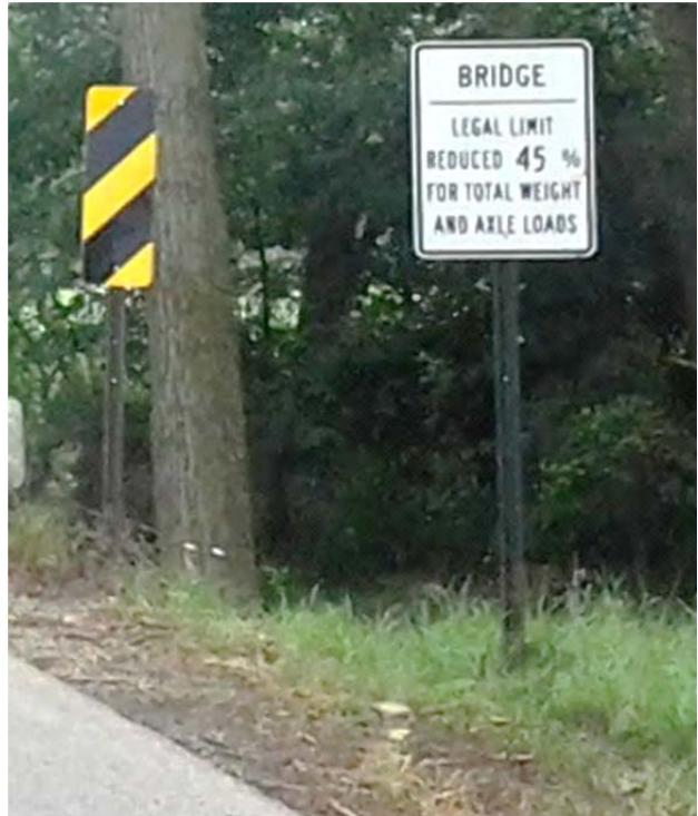
Figure 17 – Example of % Reduced Sign. % Signs were Removed from the OMUTCD January 1, 1997
