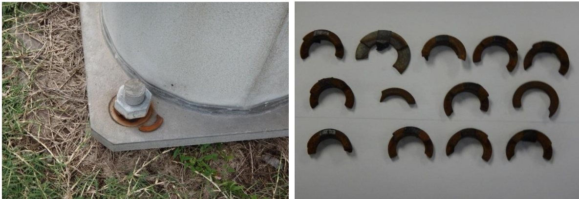
Figure 6.11 (Left) Cracked washers; (Right) Cracked washers collected by District 12
