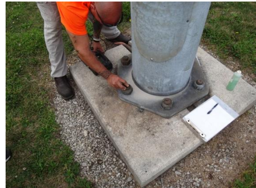
Figure 6.1 UT inspection of anchor bolts (District 2)
