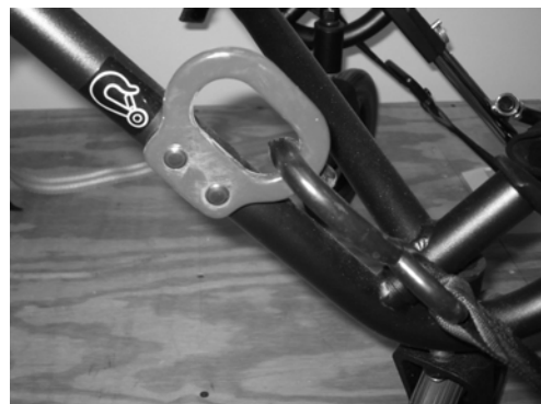
Detail of WC-19 “Transit Option” loop and labeling >
