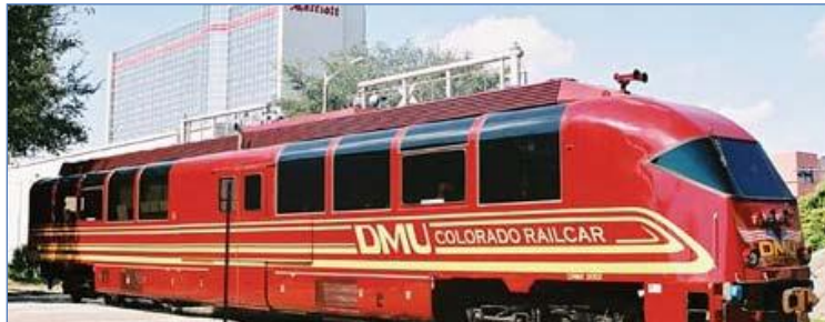
Exhibit 10-11 FRA Compliant DMU Vehicle
