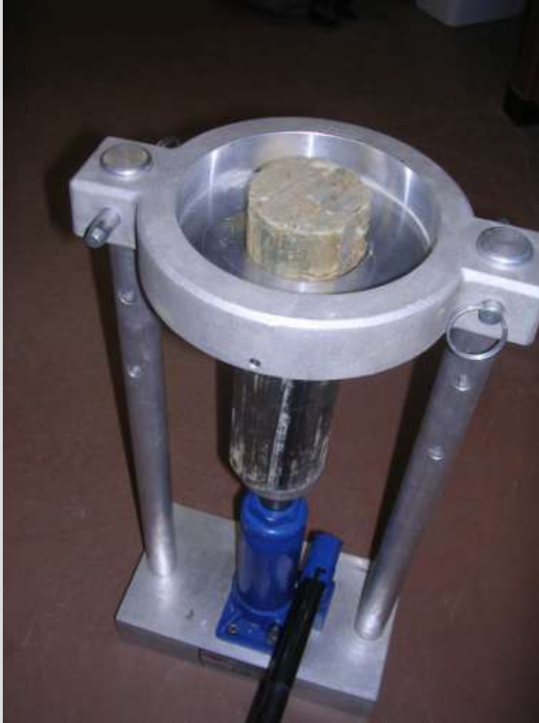
Hydraulic Jacking of Soil Sample Out of Shortened Shelby Tube
