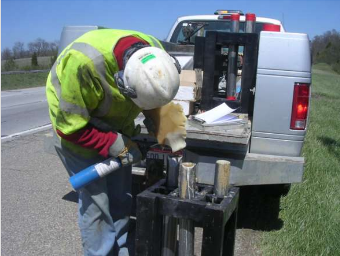
Sealing of soil sample by melted wax
