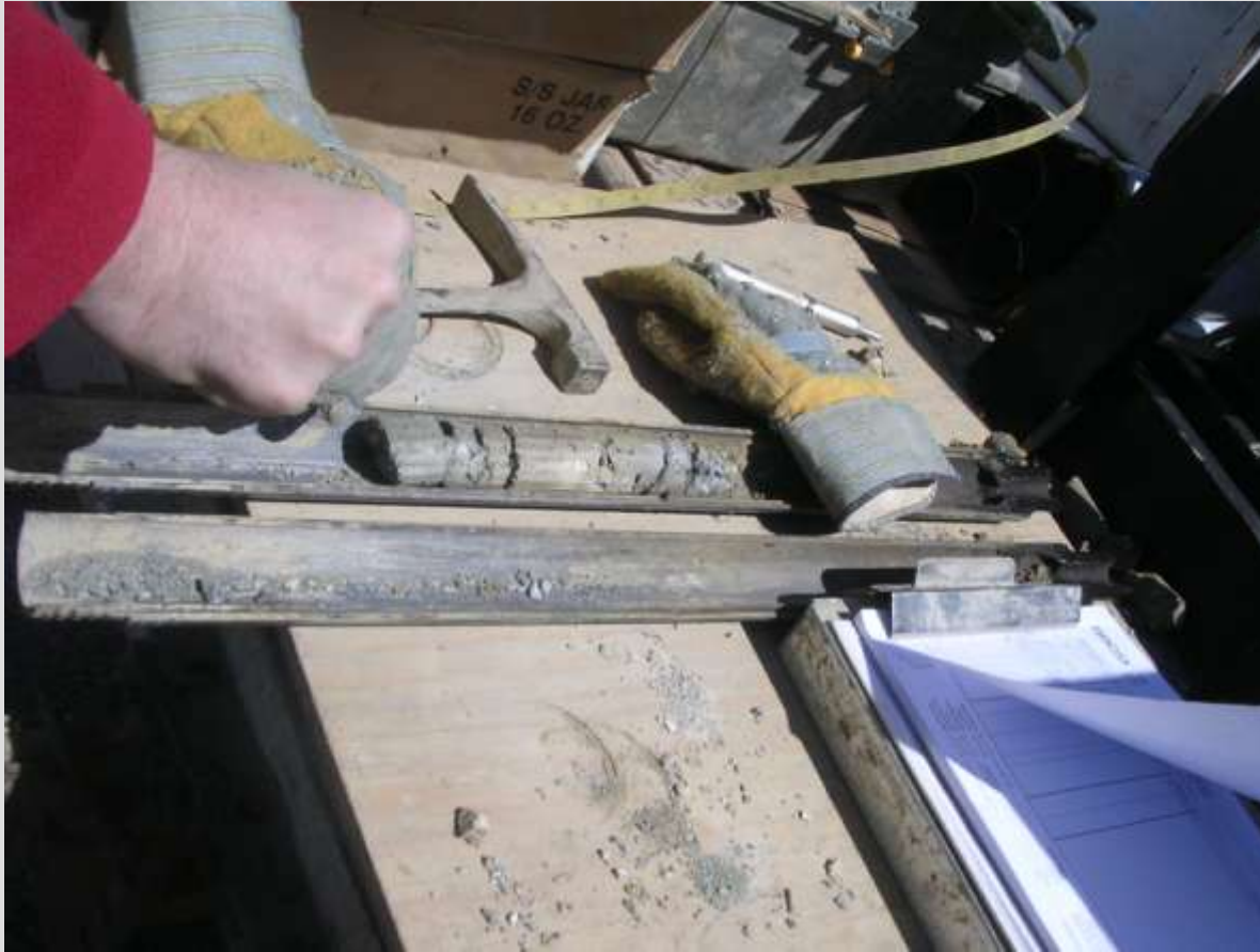
Logging of soils by split-spoon sampler
