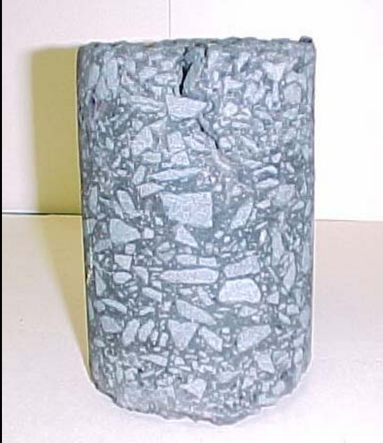
Top Down Cracking
