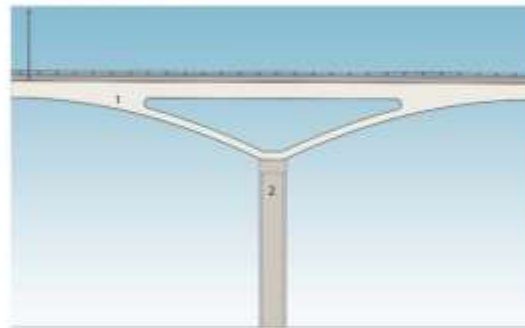
MAIN SPAN PIER SIDE ELEVATION (PIERS 3-11)
