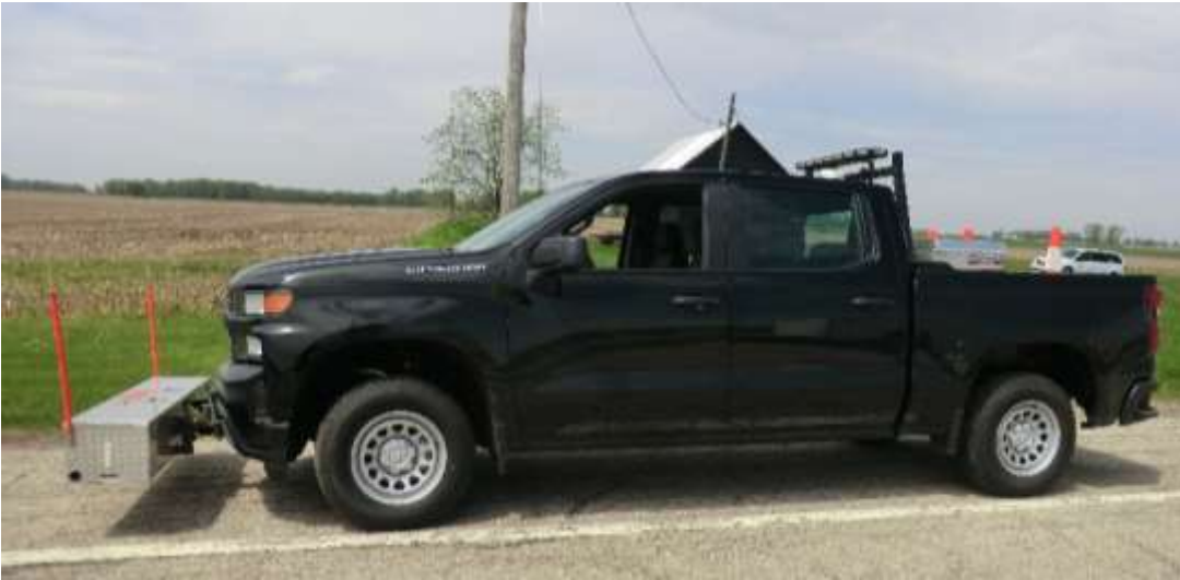
Gerken Paving Inc. Approved Road Profiler: Device 26
