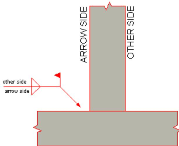
In the figure above a field welded fillet weld is required on both sides of the “T” joint. The welding symbol on the bottom of the reference line indicates a weld on the arrow side (the side of the joint that the arrow is pointing to). The welding symbol on the top of the reference line indicates a weld on the other side (the side of the joint opposite of where the arrow is pointing). The solid triangle (or flag) indicates the weld is to be made in the field.
