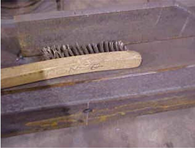
All unpainted surfaces to be welded have to be free from all loose or thick scale, slag, rust, moisture, grease, or other foreign material by Code. Mill scale that can withstand a vigorous wire brushing, or anti-spatter compound may remain prior to welding.
