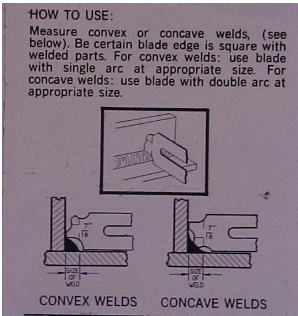
The profile of the welds should be checked. The AWS D1.5 Bridge Welding Code shows acceptable and unacceptable weld profiles. These are shown below:
