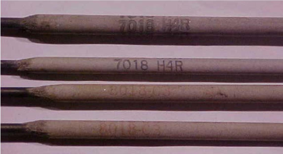
E7018 electrodes are used for bridge members that are coated (painted, galvanized, or metalized).
