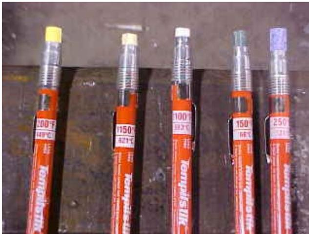
If the weld joint has reached the required level of preheat the appropriate Tempstick will melt when rubbed across the base metal
