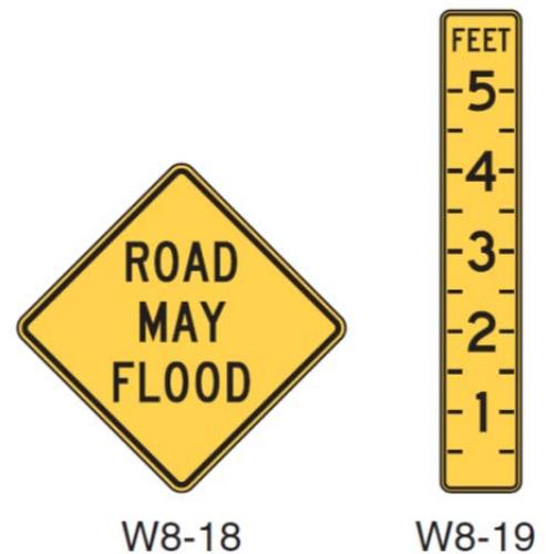
Figure 34 - Flood Inspection Signage
