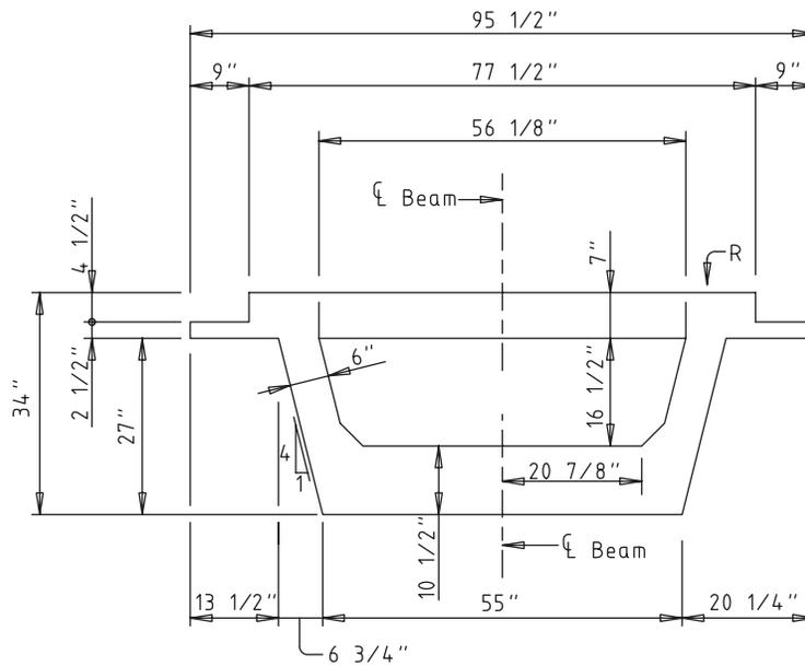
FIGURE 3 Typical pretopped U-beam section.
