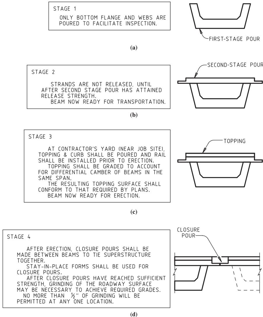
FIGURE 5 Pretopped U-beam construction sequence.
