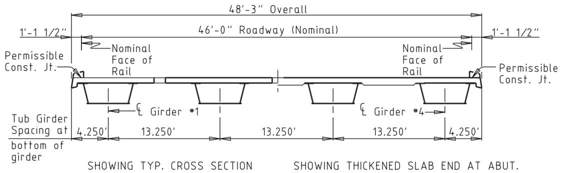
FIGURE 2 Steel girder superstructure.
