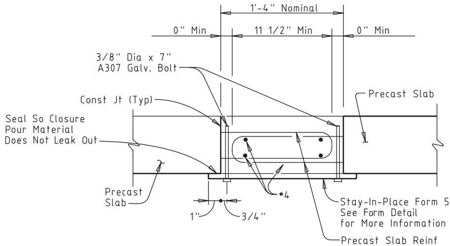
FIGURE 6 Steel tub-girder longitudinal closure pour detail.
