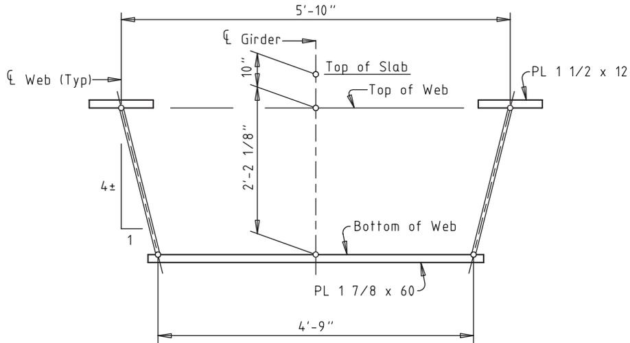
FIGURE 1 Typical steel girder section (PL = plate).
