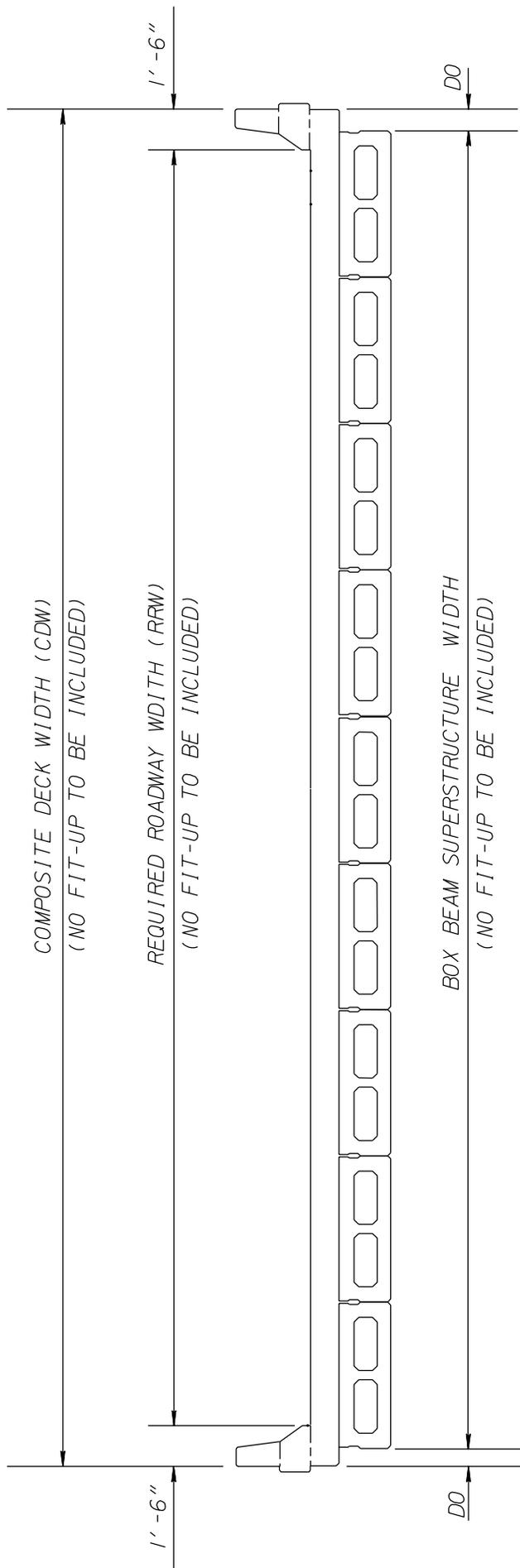
*FIT-UP SHOULD NOT BE INCLUDED IN ESTABLISHING THE NUMBER OF BEAMS.
