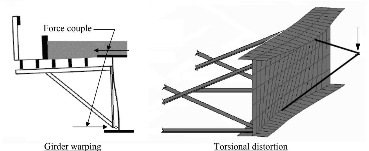
For steel superstructures, Designers should calculate the magnitude of twist ( $\mathbf{N}_w$ ) due girder warping using the TAEG software developed by the Kansas Department of Transportation. TAEG (“Torsional Analysis of Exterior Girders”) is available at no cost and can be downloaded at: <http://www.ksdot.org/kart/>.
