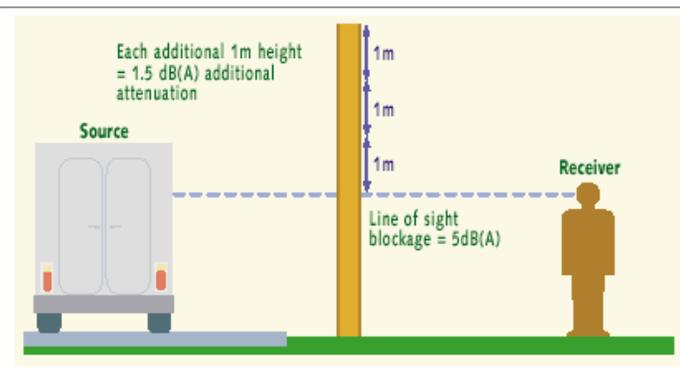
To effectively reduce the noise coming around its ends, a barrier should be at least eight times as long as the distance from the home or receiver to the barrier.
