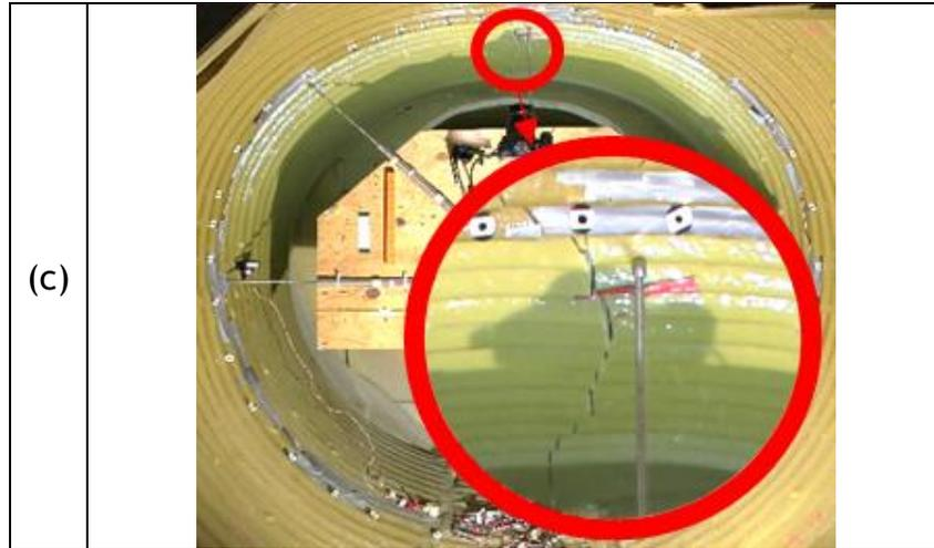
Figure 11-60. Formation of the first structural crack. It shows (a) 0.25 in. SAPL renewed circular CMP at 39 kips, (b) 0.5 in. SAPL renewed circular CMP at 42.78 kips, and (c) 1 in. SAPL renewed circular CMP at 66.26 kips.
