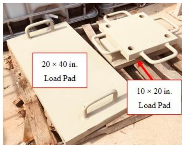
Figure 11-19. Steel load pads.
