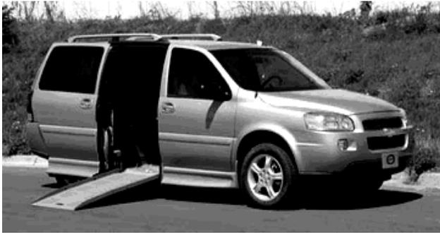
This vehicle is a standard production minivan modified by lowering the floor and, in some cases, modifying the roof at the entryway to provide the 58" headroom required by ADA. It is the smallest accessible vehicle available, accommodating up to two wheelchairs and one permanent seat, with an option for quick-release seats for three additional ambulatory persons in the wheelchair securement locations.
