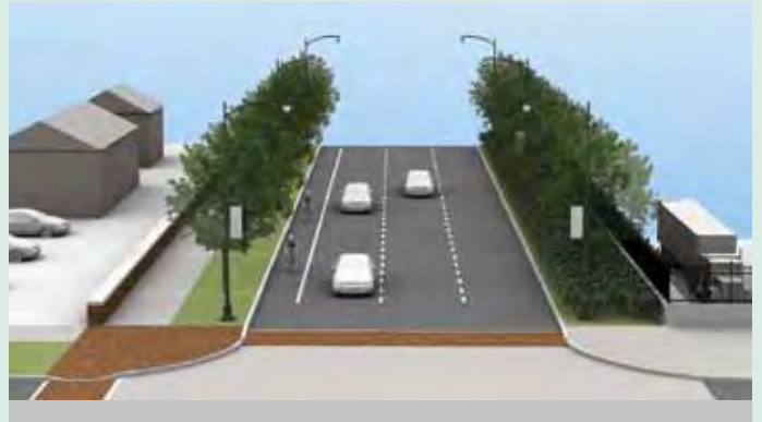
Lester Drive Cross Section (Spring St. to Broad St. shown)
